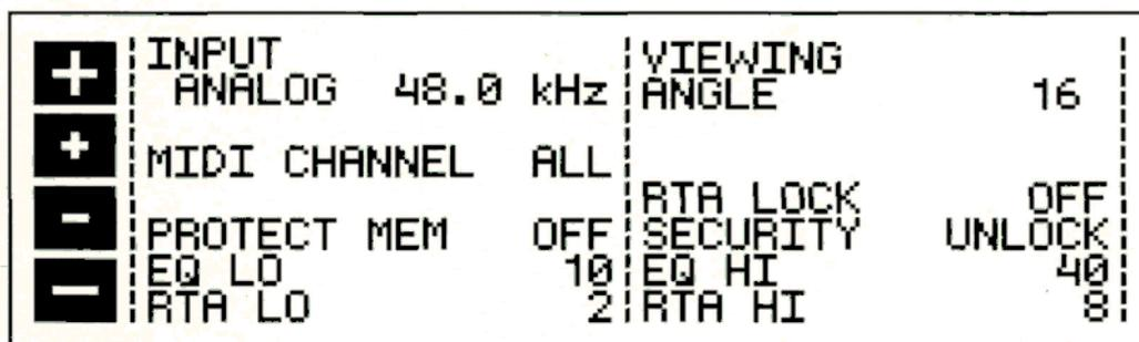
Fig. 6.1: Configuration Window in the ULTRA-CURVEs GENERAL SETUP menu
